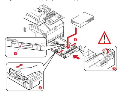
**4.** Adjust the rear stopper and paper guides (2) to the size of paper being used.
